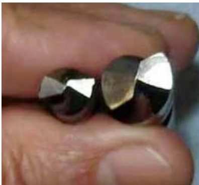
Thinning of web is recommended on larger drills
