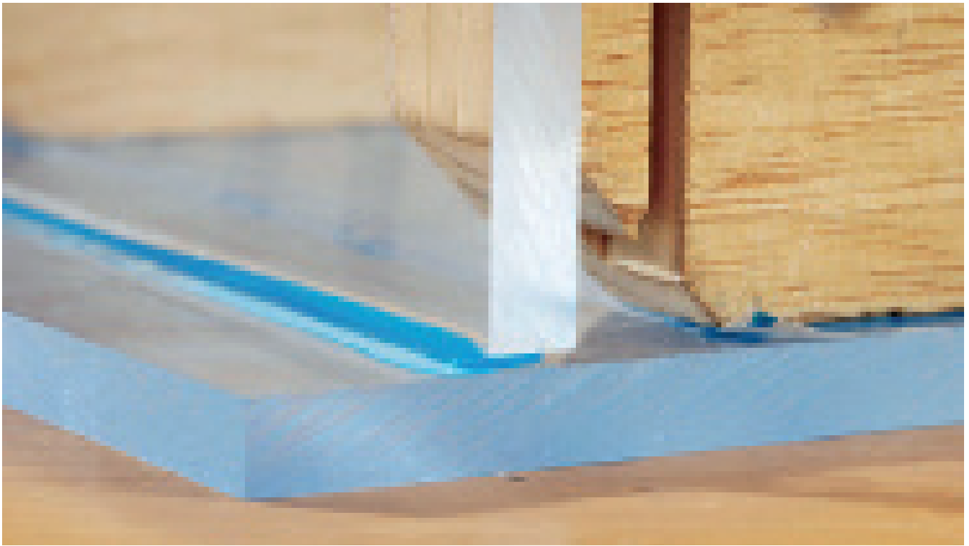
ACRIFIX® 1R 0192 seeps into the joint area on its own.
