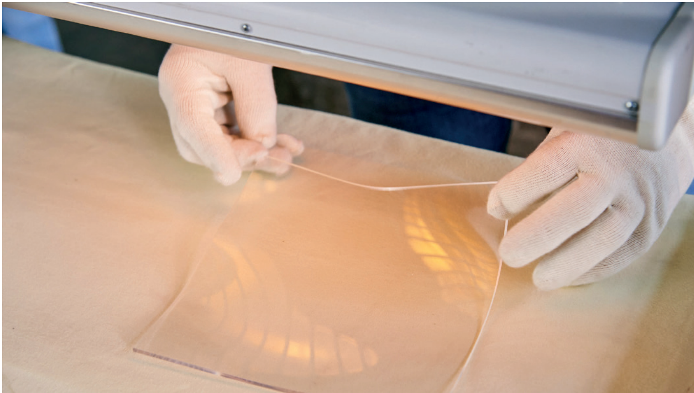
The cut-to-size PLEXIGLAS® sheet is placed under the bath radiator for heating.
