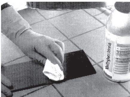
Figure 13: Chemical treatment of a previously sanded surface
