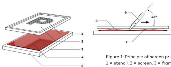
Figure 1: Principle of screen printing
