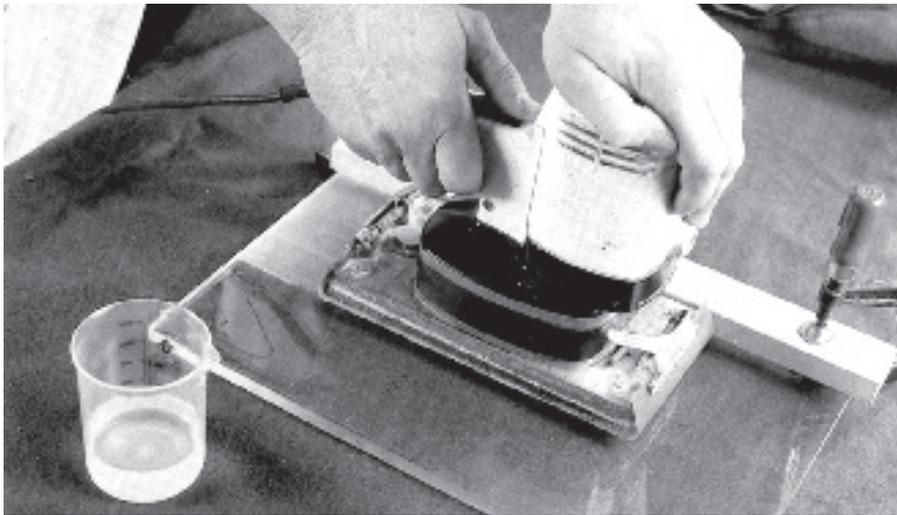
Figure 11: Mechanical matting with an orbital sander
