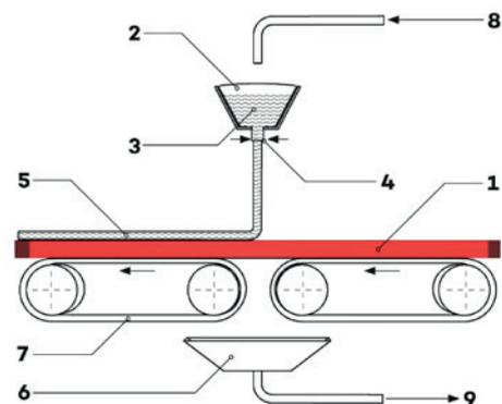
Figure 9: Principle of flow coating
