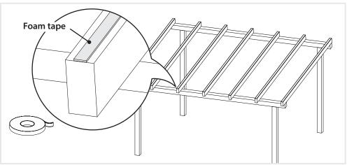
Applying foamed tape on each rafter will reduce friction due to thermal expansion.
