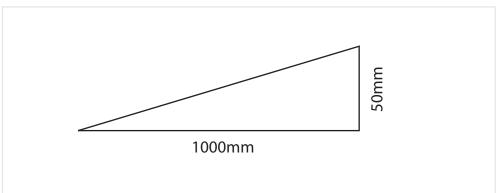
• To ensure proper water runoff, slope should be at least 5% (50mm rise over 1m length).
