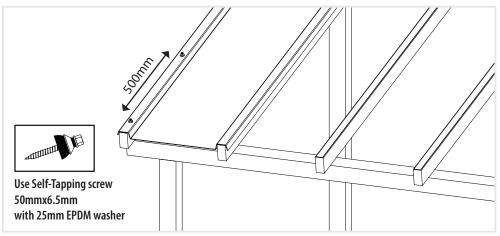
Fix the first EZ Glaze panel's outer corrugation, using specified screws and washers through the pre-drilled holes. Start at the bottom edge and work your way up.
