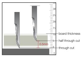
We use a ZÜND M250 cutter, the setting may vary when using other cutting machines.
